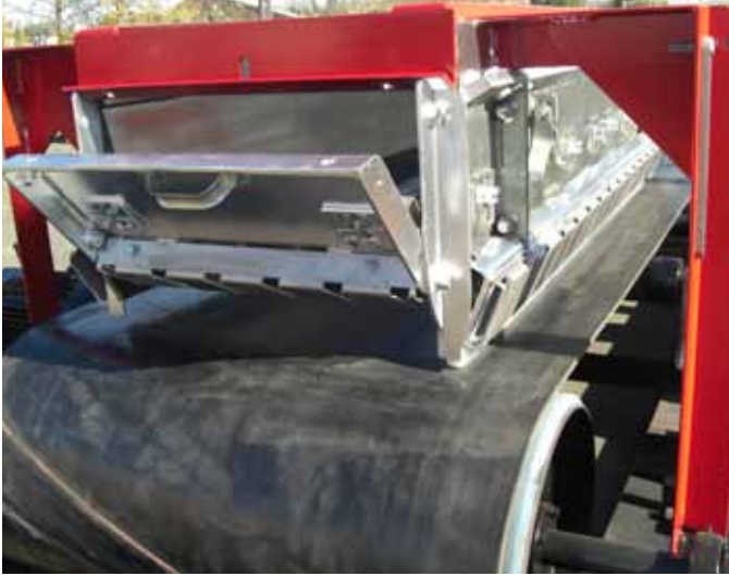
Pivoting EZ-ACCESS™ Taildoor can be custom specified or field fabricated to size on sight.
