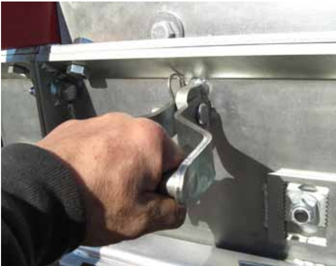
Pin-on lifting handles can be used for handling or opening doors.
