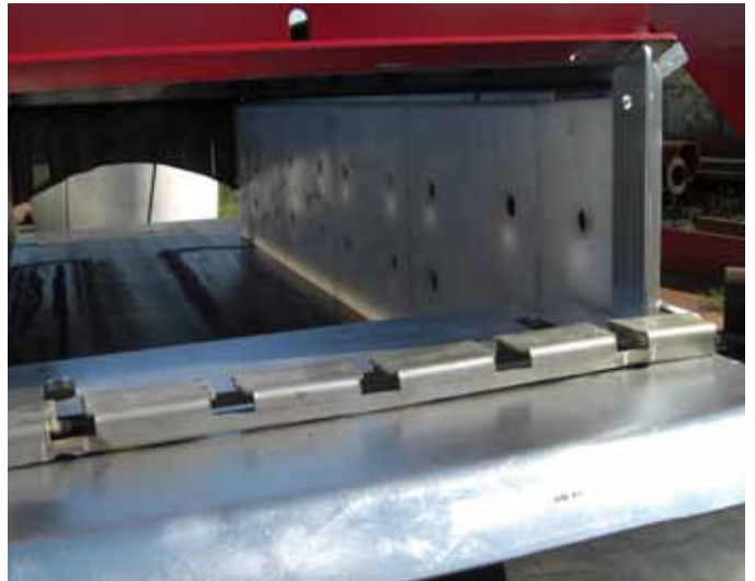
Pin-on EZ-SKIRT® hanger without flexible inner tailskirt shown inside of tailbox. UHMWPE liners shown on unit.
