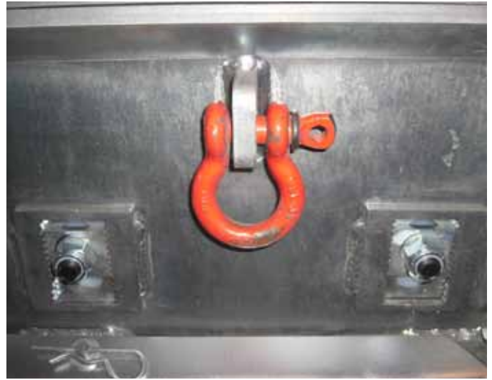
Clevises may be inserted into padeyes for lifting individual doors or assemblies.
