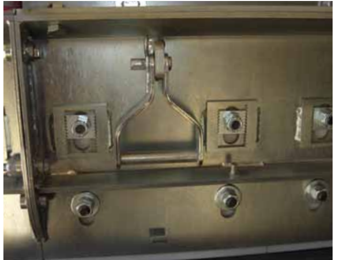
Wear Liners include 4 fasteners per liner. The EZ-ACCESS™ System comes standard with the patented LINERLOCK™ system for secure attachment and precision adjustment.
