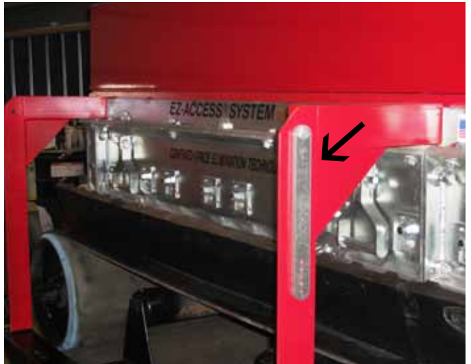
Safety Lockout Bars kept handy available for quick access during maintenance for Tall and Standard units. (Tall shown)
